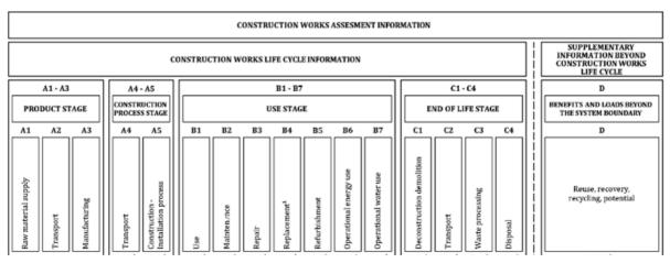
Figure 8: Scheme for sustainability assessment of construction work according to EN 15804:2019.
