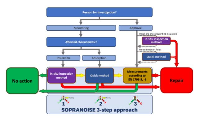
Figure 7: Flow chart visualizing the scope of the SOPRANOISE 3-step approach (see report D5.2 and D3.1 of SOPRANOISE).
